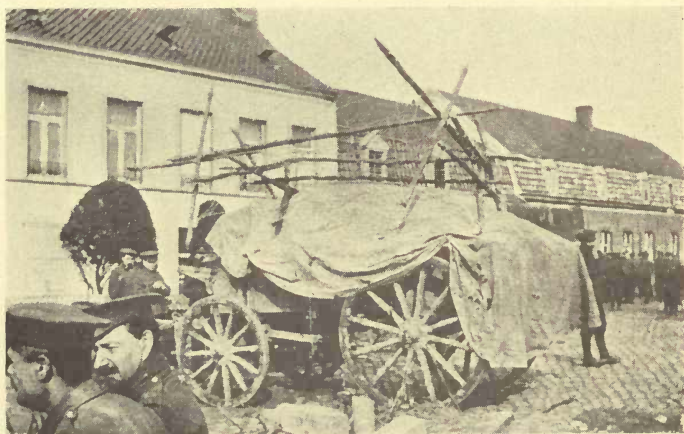
THE PRINCESS PATRICIAS IN BILLETS AT WESTOUTRE, BELGIUM. ON TOP OF WAGON IN FOREGROUND IS "KNIFE-REST" TYPE OF WIRE ENTANGLEMENTS.
